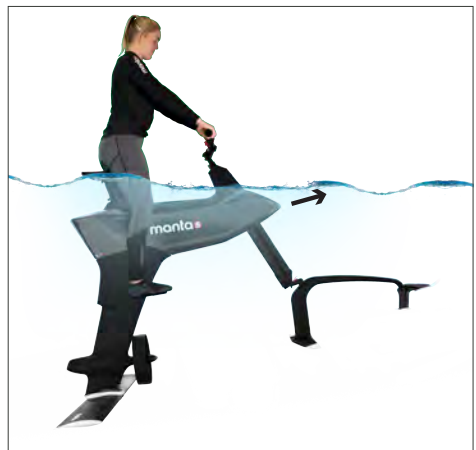
7.4 Once you are comfortable riding underwater at maximum throttle you can begin to slowly lean back. As you lean back you will feel the take-off. Think aircraft taking off on a runway. The heavier you are the longer your runway needs to be.
