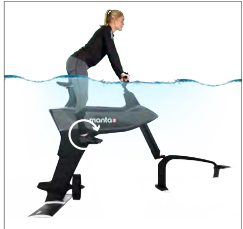
7.2 Stand on the pedals whilst staying in an upright position and rotate the pedals one full rotation to activate the motor, allowing the throttle to become active.
