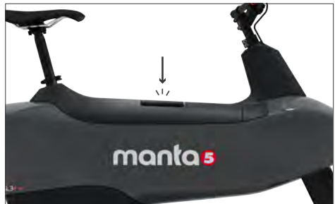
5.4 Next, push the handle down locking the battery into place. An audible click can be heard once connected correctly. Your bike is now ready to be carried to the water.
