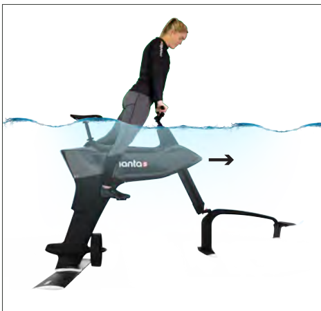
7.3 First time riders are encouraged to get comfortable riding on the bike completely submerged. Do not attempt to launch right away. Do this for a minute until you can feel the pitch of the bike increase as you throttle faster and faster until you are at maximum throttle. Practise leaning your chest over the handlebars to control the launch angle.
